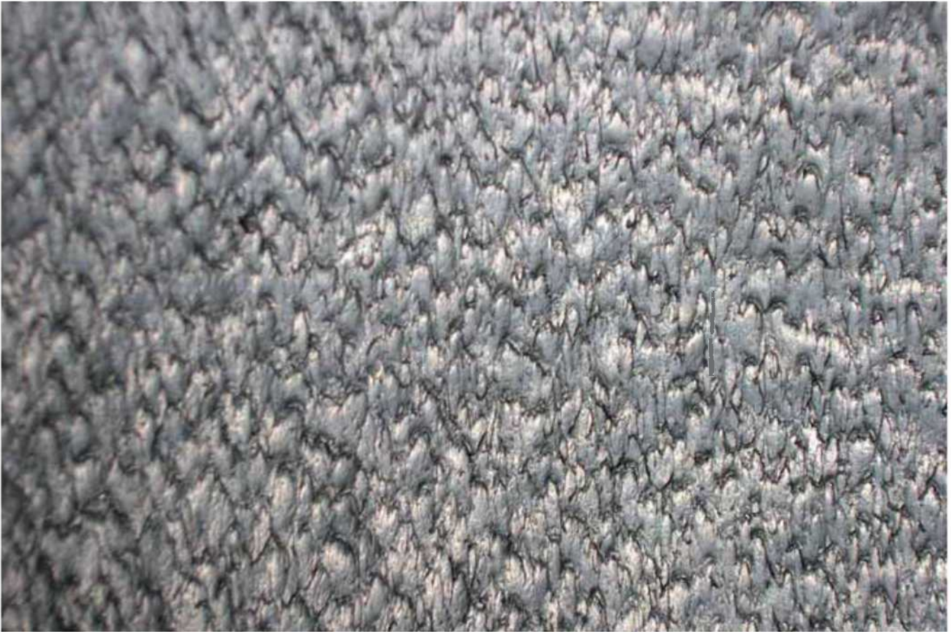
Figure 5 | Coextruded surface texture (blown-film process)
