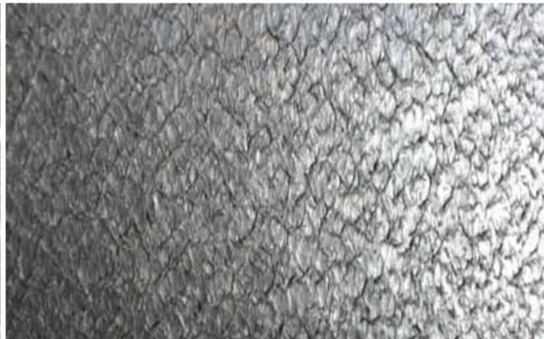
Figure 4 | Coextruded surface texture (blown-film process)
