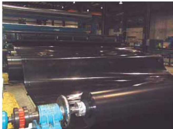
Figure 1 | Flat-die calendaring manufacture (smooth-sheet production)
