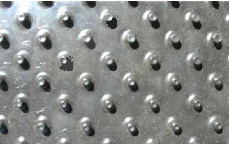
Figure 3 | Flat-die molded structured surface (drain-surface profile)
