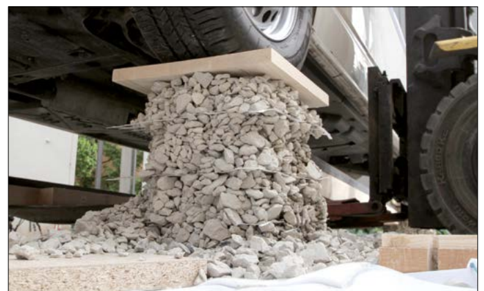
Fig. 2 Demonstration of the interlocking effect under a 2.2t van
