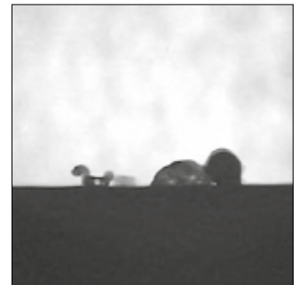
Figure 2: Visual comparison of embossed structure (A, left), co-extruded structure (B, middle) and sprayed structure (C, right)
