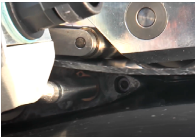
Figure 2: Close-up of heated wedge
