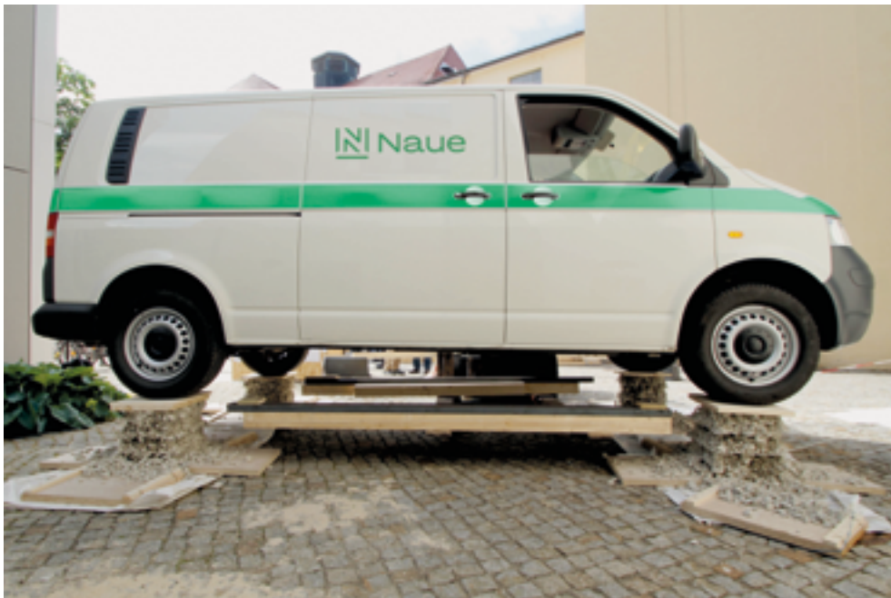
Figure 2: Secugrid® geogrid reinforced stone columns carry a nearly 2-ton heavy delivery van during a live experiment (see the following QR-Code)
