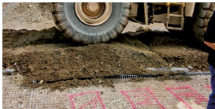
Figure 15: Installation damage factor (" RF_{ID} / A_2 ") determined by a field trial in a quarry
