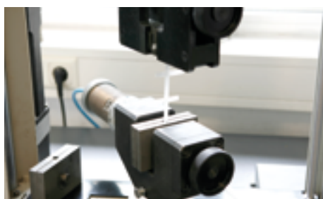
Figure 17: Junction strength test using a Secugrid® geogrid sample
