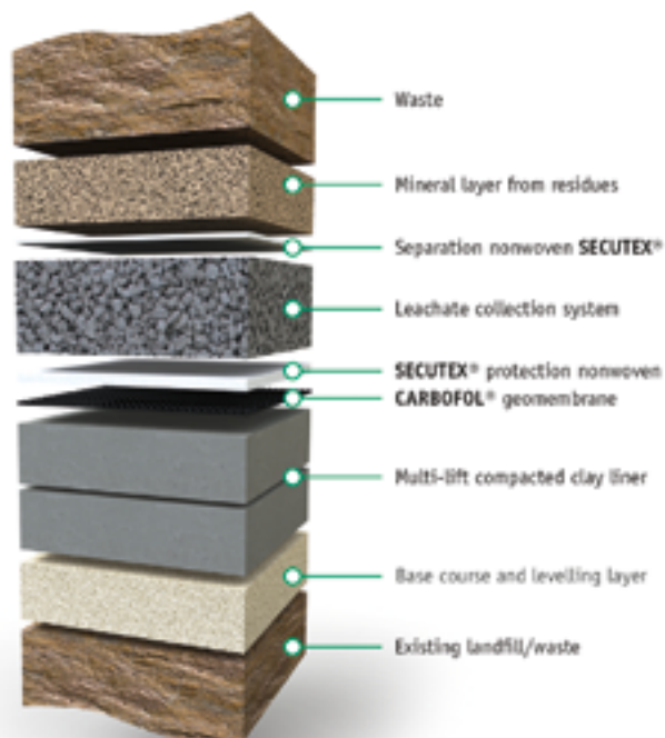
Figure 2: Intermediate sealing system for municipal solid waste landfills
