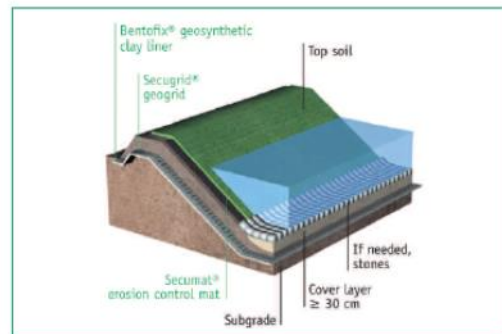
Figure 3 Secumat® as erosion control on a dike or storm water retention pond
