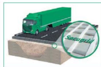
Figure 4 Secugrid® reinforcement over areas prone to subsidence
