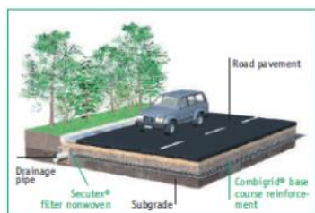
Figure 7 Base course improvement with the composite product Combigrd® for separation and reinforcement
