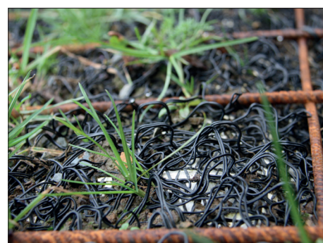
Figure 12: Secumat® 601 40/ 40 Q6 with initial vegetation
