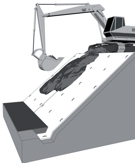
Fig. 10 Adding the soil using machinery
