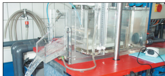
Determination of water flow capacity in their plane (EN ISO 12958)
