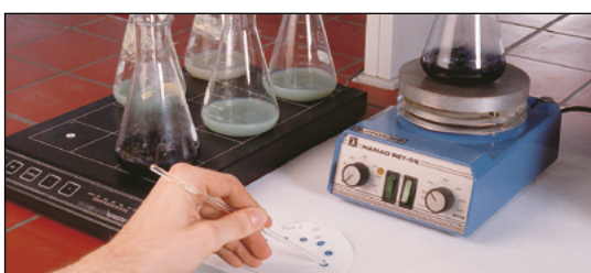
Determination of the montmorillonite content of bentonite via the methylene-blue-adsorption (titration) method (VDG P69)
