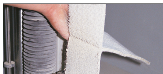
Determination of the bonded peel strength of Bentofix® geosynthetic clay liners (ASTM 6496)
