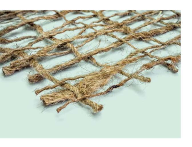
**Secumat® Green Jute N** is a sustainable, temporary erosion control solution. It comprises a warp (vertical) and weft (horizontal) woven net with displaceable openings in the net. It is made from 100% untreated jute fibres which have a natural variance in thickness when spun and is completely biodegradable.
