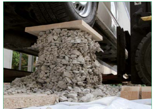
Figure 7: Interlocking effect demonstrated by a Secugrid® reinforced gravel column supporting a van
