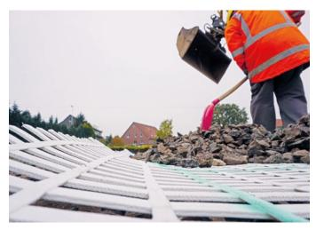
Figure 4: Field trial with Secugrid® HS to determine the installation damage  $(RF_{CR})$  reduction factor
