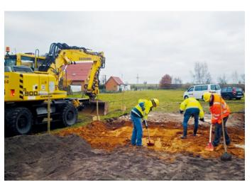
Figure 5: Uncovering of Secugrid® HS to determine the installation damage (RF<sub>CR</sub>) reduction factor
