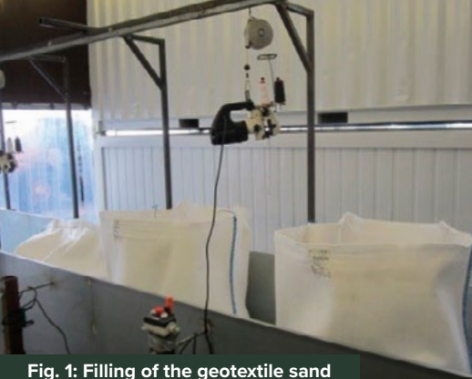
Fig. 1: Filling of the geotextile sand containers
