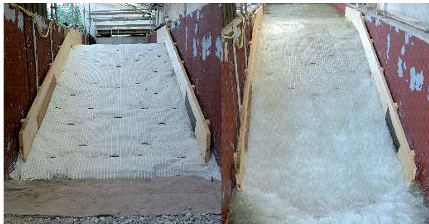
Fig. 12 Model experiments at the Technical University Munich, Overflow of the inner embankment per method (II) Left: before overflow, right: in overflow state with up to 300l/m-s (Haselsteiner et al. 2007)
