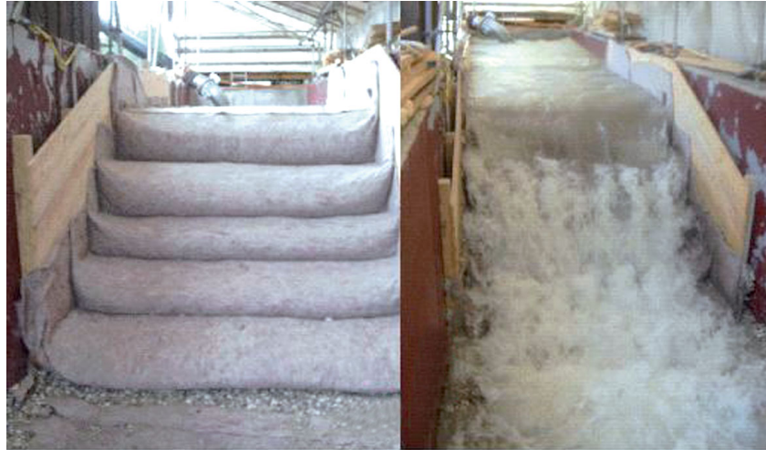
Fig. 11 Model experiments at the Technical University Munich, Overflow of the inner embankment per method (III). Left: before overflow, right: in overflow state with up to 130l/m-s (Haselsteiner et al. 2007)
