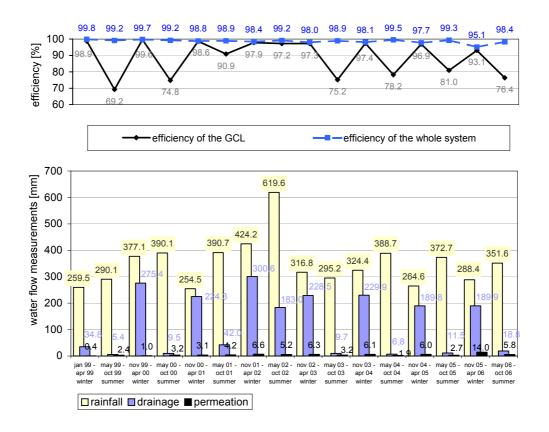
Figure 4. Lysimeter 3 – effects of summer and winter cycles on the sealing efficiency of a single-layer, standard Bentofix<sup>®</sup> bentonite mat with a 1-m recultivation layer
