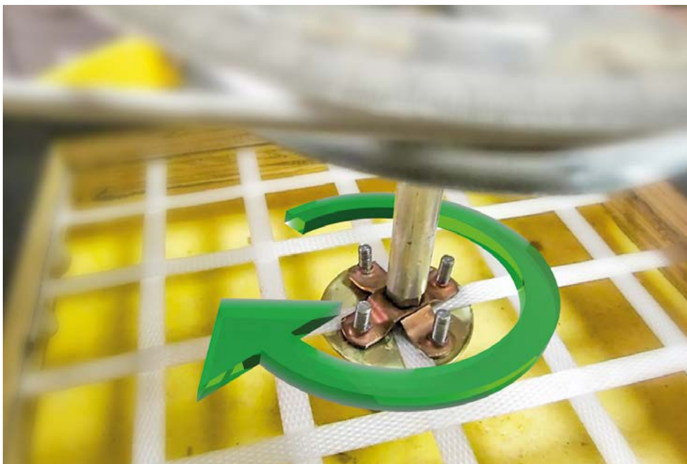
Figure 13: Application of torsional stress to Secugrid® geogrid sample in a test rig
