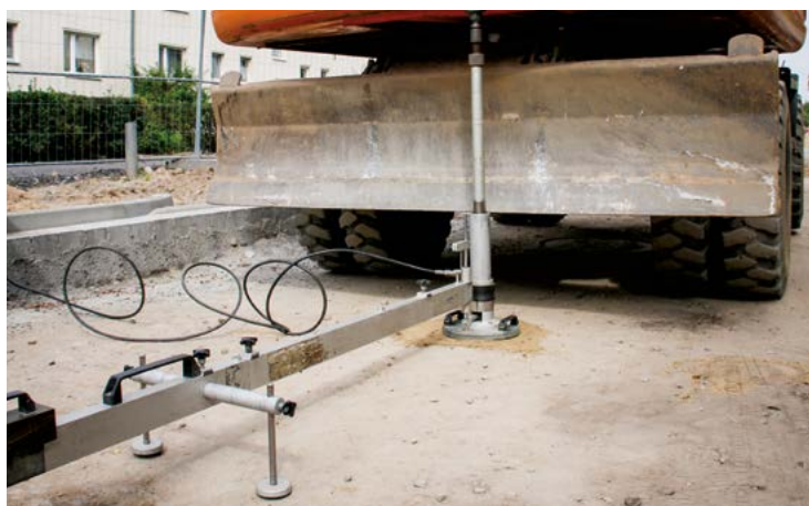
Figure 19: Plate bearing test according to DIN 18134 using a 300mm diameter load plate
