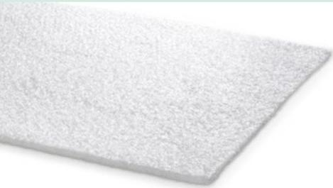
Since the early 1960s, nonwoven geotextiles have been used in various fields of civil engineering for separation, filtration, protection and drainage applications. Since then, numerous national and international guidelines have been published that enable project-specific specifications and product selection, based on established performance requirements.
