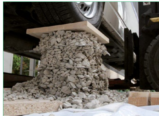
Figure 7: Interlocking effect demonstrated by a Secugrid reinforced gravel column supporting a van
