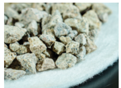
Figure 11: Secutex® as protection against, e.g., drainage gravel
